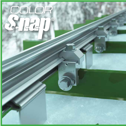
Color Snap® Installation 9/16" Hex Bolts w/Rail Connector (190 in-lbs)
