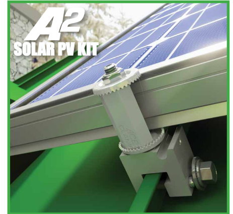
A2 SOLAR PV KIT Solar PV Kit Installation Kit Mounting Post - 3/16" Hex Drive (100 in-lbs) 9/16" Hex Nut securing PV Panel (100 in-lbs) max
