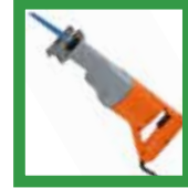
Sawzall to trim excess length of rail
