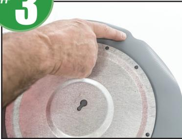
Position the MCP over the head of the fastener and slide as shown.
